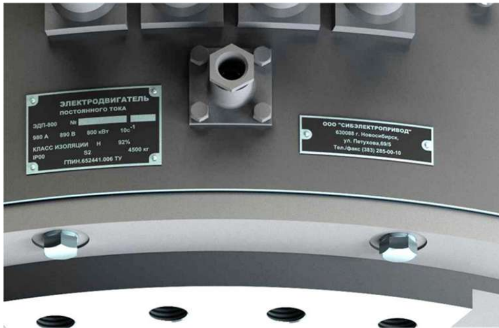
Figure 8 – Example of the traction motor labeling
