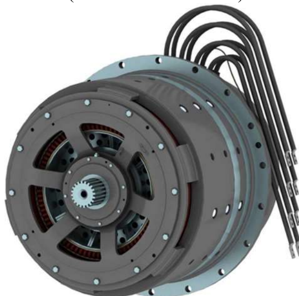
Figure 1 – Design of EDP-800 traction motor (commutator-side view)
