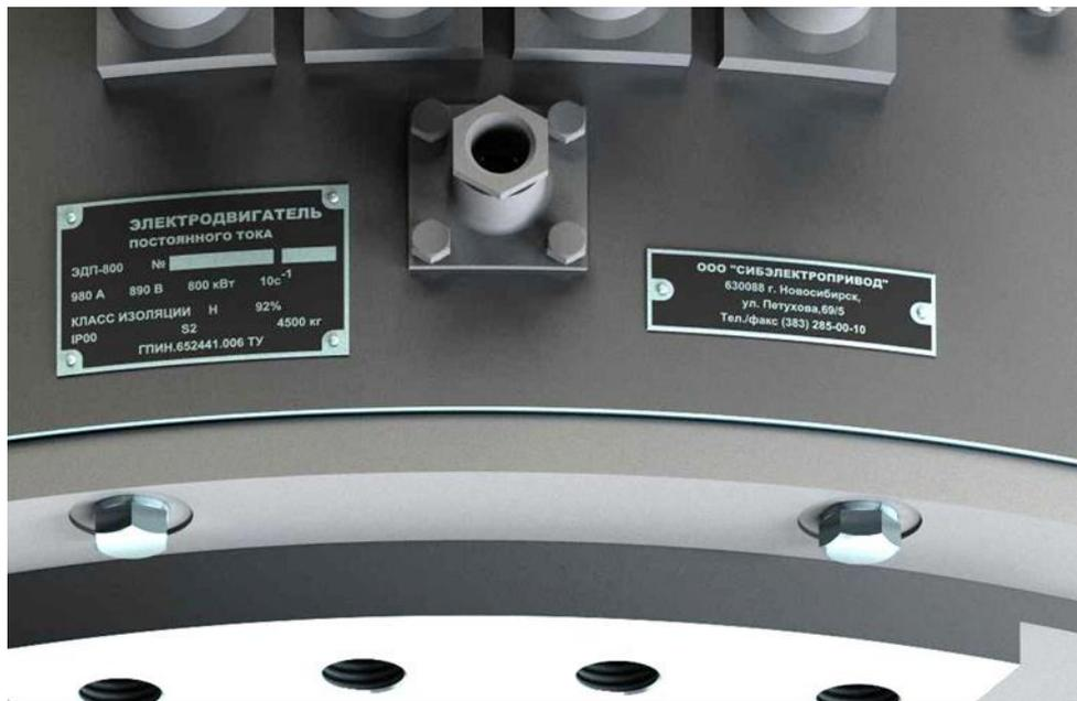
Figure 8 – Example of the traction motor labeling
