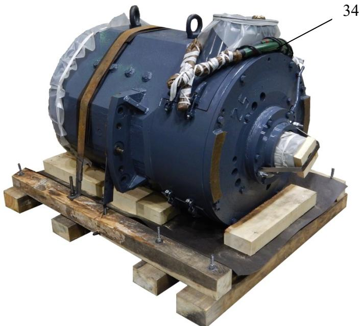
Figure 9 – Example of the traction motor packing
