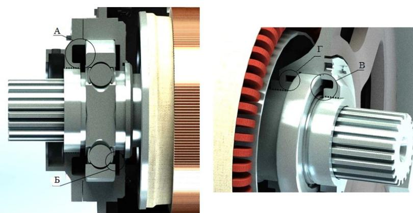
Figure 18 – Replenishment of lubricant in bearing assemblies
