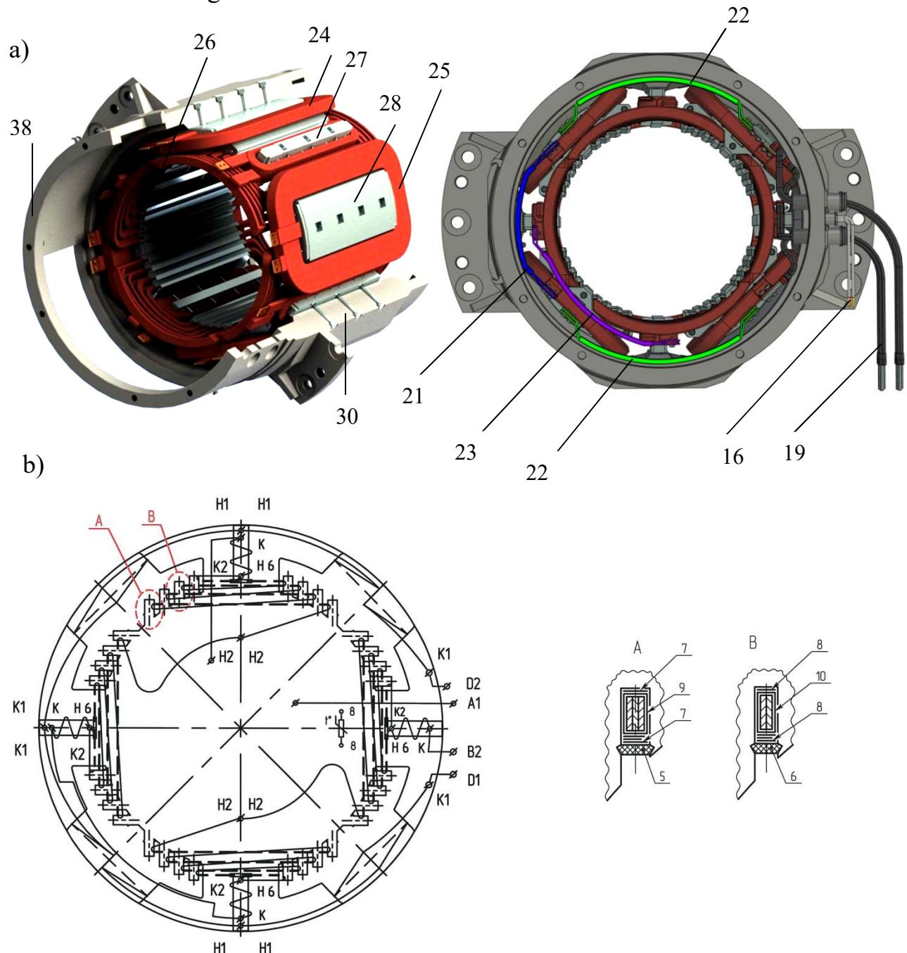
Figure 4 – a) magnetic system of the traction motor b) windings electrical connection diagram
