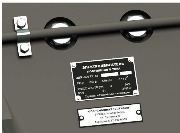
Figure 8 – Example of the traction motor labeling
