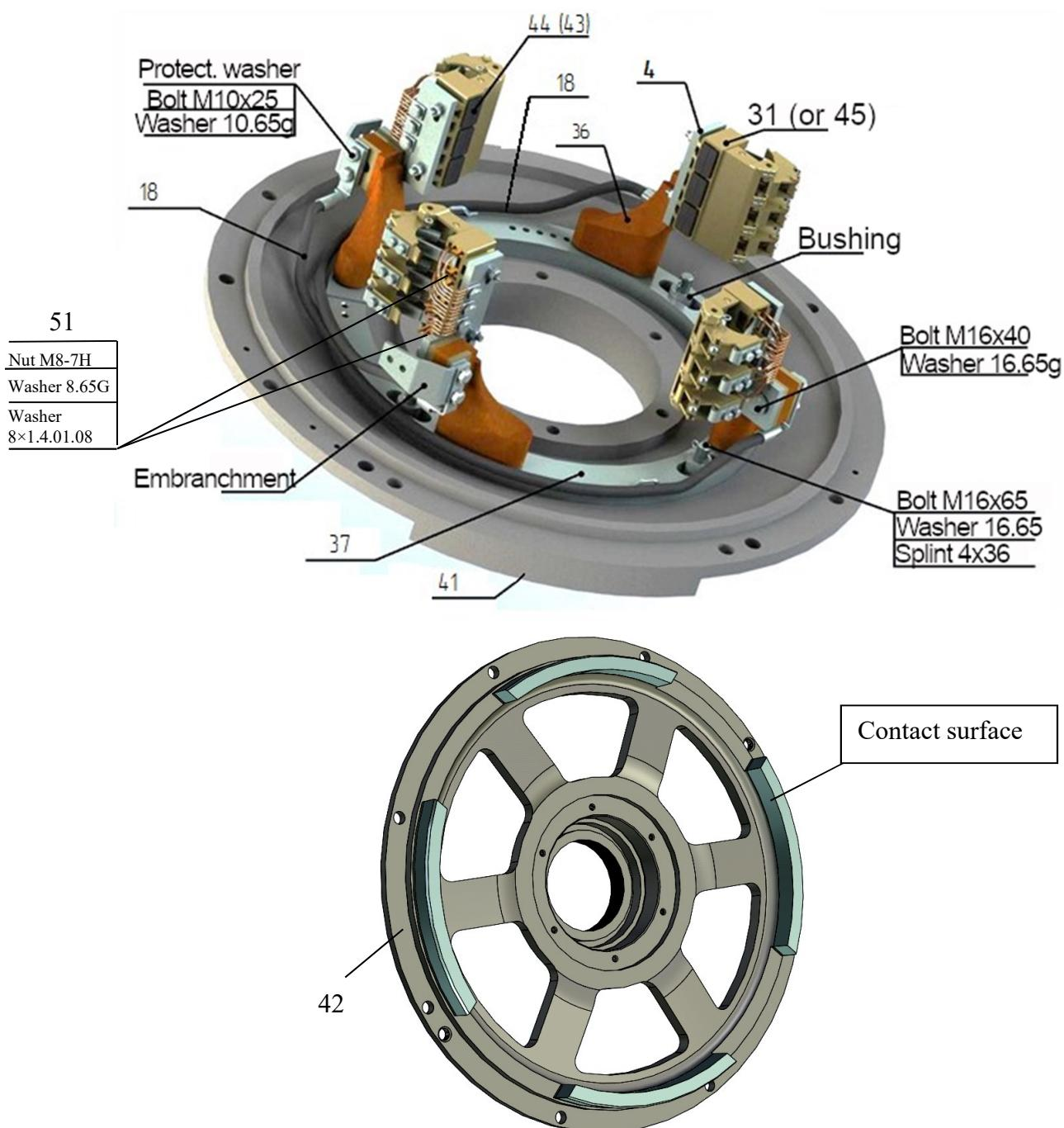
Figure 6 – End shield of the traction motor
