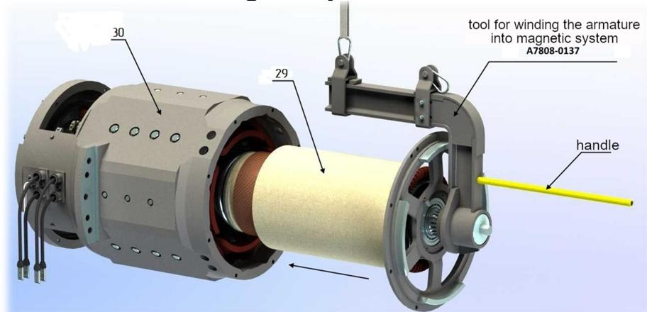
Figure 19 - Winding the armature into the magnetic system
