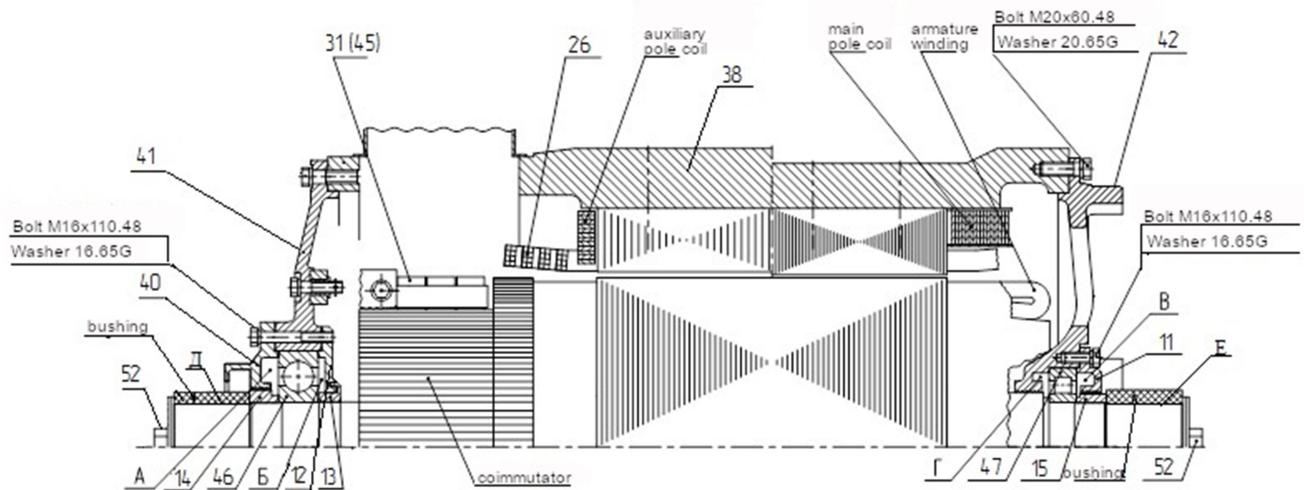
Figure 15 – General view of the traction motor EDP-600
