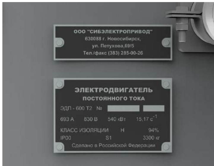
Figure 8 – Example of Electric Motor Marking
