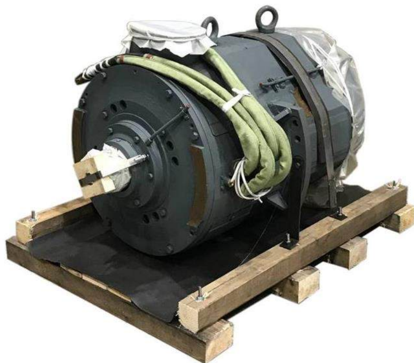
Figure 9 – Example of Lightweight Packaging for the Electric Motor (external protective film removed).
