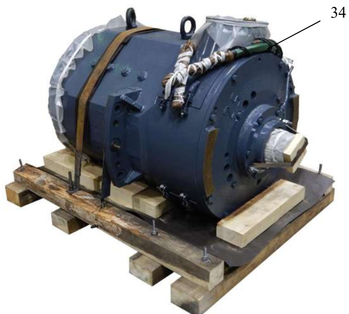
Figure 9 – Example of the traction motor packing
