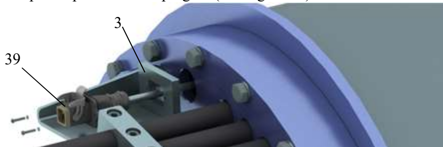
Figure 10 – Dismantling of the Connector
