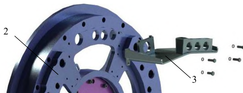
Figure 35 – Installation of Holder
