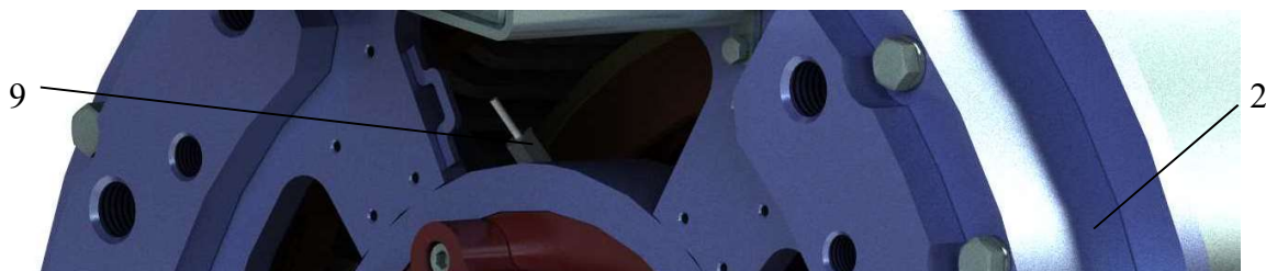
Figure 48 – Installation of Bearing Temperature Sensor on the Brake Side
