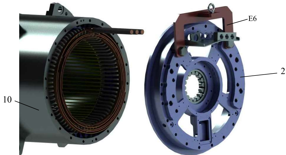
Figure 24b – Dismantling of the Bearing Shield (Brake Side)
