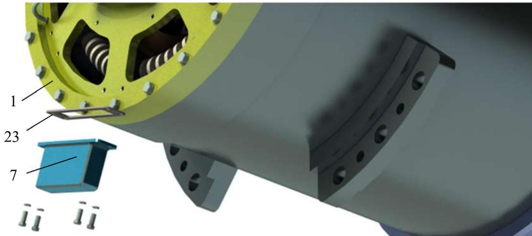
Figure 51 – Installation of Oil Pan for Waste Grease
