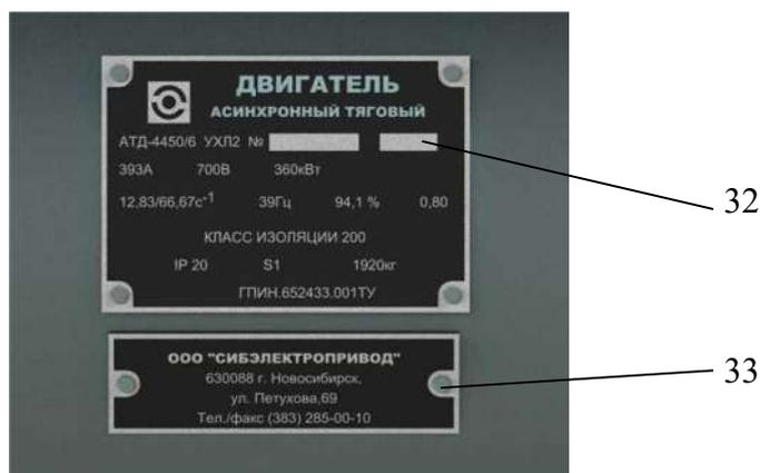
Figure 7 – Example of Motor ATD-4450/6 Marking
