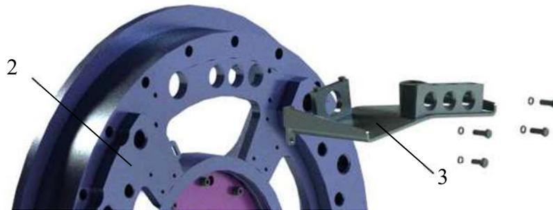
Figure 35 – Installation of Holder
