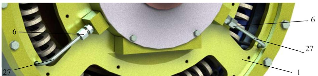
Figure 45 – Installation of Tubes for Grease Replenishment
